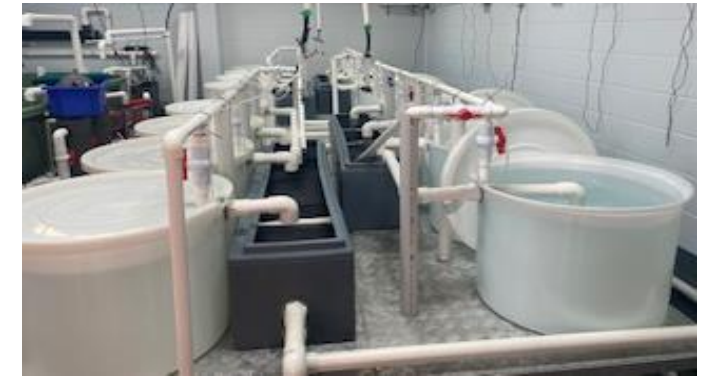
Disease challenge test system - 4 systems with 4 tanks per system: IHHNV, GAV, YHV-7 and control
